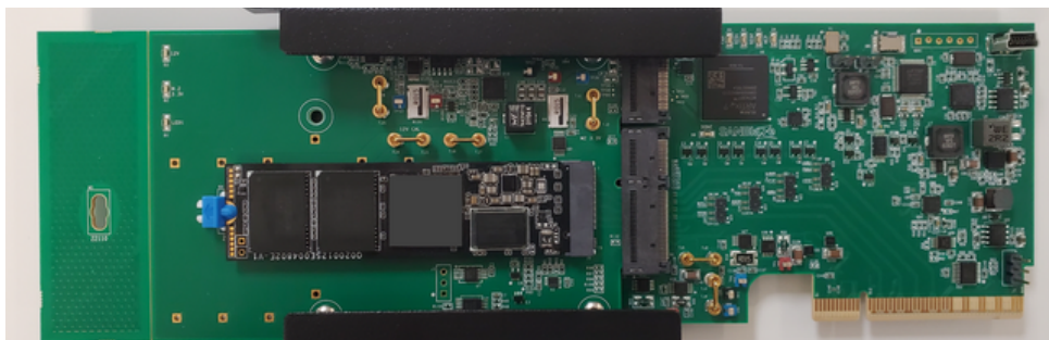
SANBlaze iRiser5+ Device - shown with optional 660 EDSFF-to-M.2 Adapter & sample M.2 SSD installed
