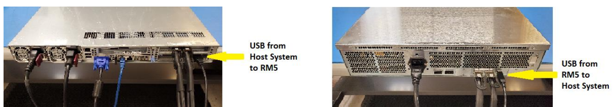
Figure 8: USB from Host to the SBExpress-RM6 NVMe System
