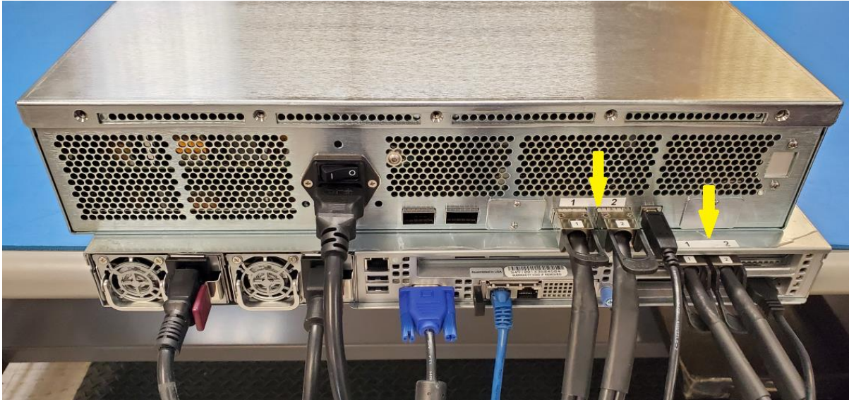
Figure 7: Connect the 2 PCIe cables from the Gen5 Host to the SBExpress-RM6 NVMe System
