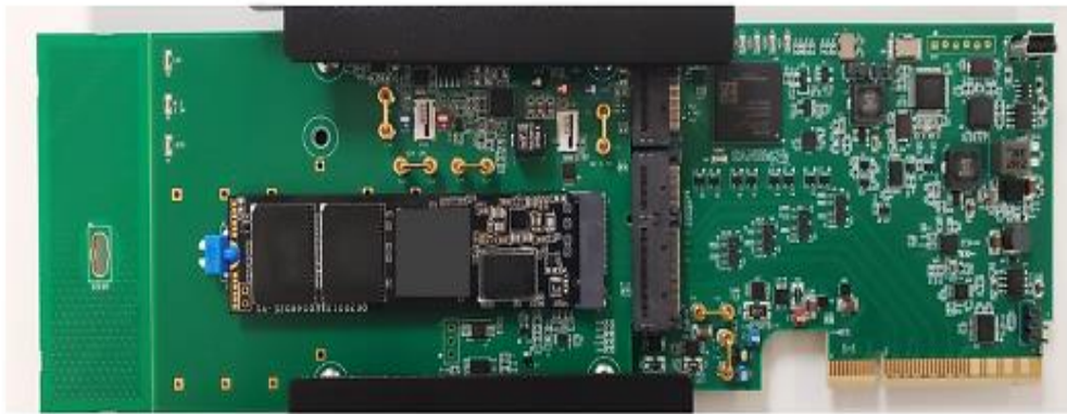
Figure 2: iRiser5+ device shown with optional 660 EDSFF-to-M.2 adapter and sample M.2 SSD installed
