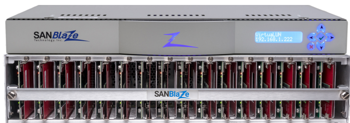
SANBlaze SBExpress-RM4 (Gen 4) Dual Port NVMe Drive Tester
